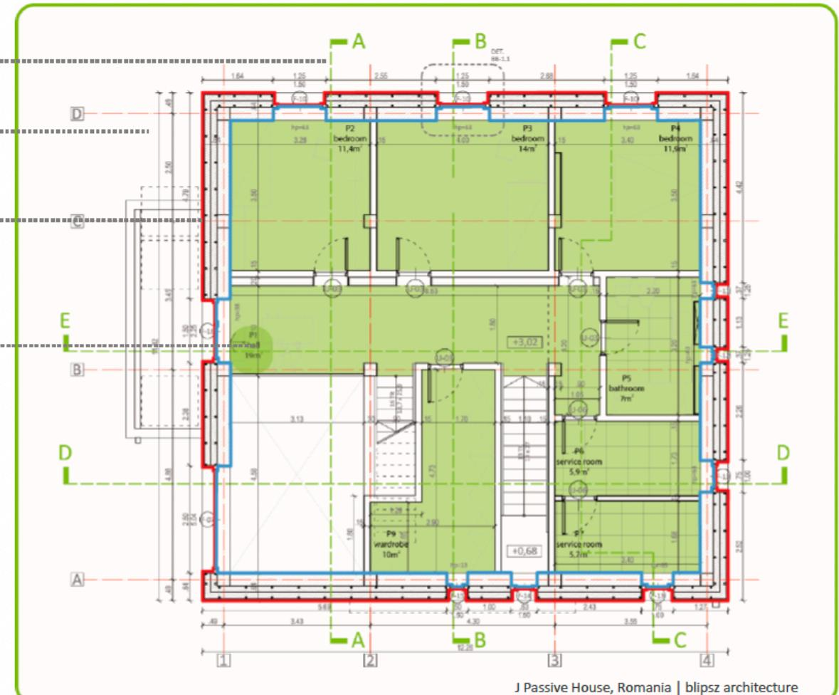
Graphic identification and external dimensions of the thermal envelope
